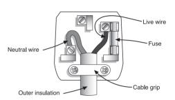
On no account must either the **BROWN** or the **BLUE** wire be connected to the **EARTH** terminal ( $\stackrel{\bot}{=}$ ). Always ensure that the cord grip is fastened correctly.
