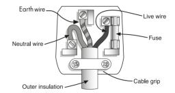
The wire coloured  ${\it BLUE}$  is the  ${\it NEUTRAL}$  and must be connected to the terminal marked  ${\it N}$  or coloured  ${\it BLACK}$ .
