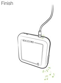
5. Once the target temperature has been reached an alarm will sound & target LED will light.
