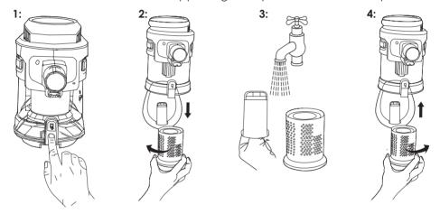
**Note:** Do not clean the HEPA filter using detergents or use external heat sources such as radiators to dry them. **Warning:** Do not reassemble or use the vacuum cleaner until the HEPA filter is fully dry, as this could cause damage.
